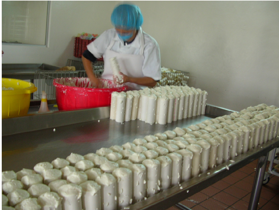
(Soft cheesemaking: placing soft goat milk cheese curds in the plastic moulds, Celaya, Mexico)
