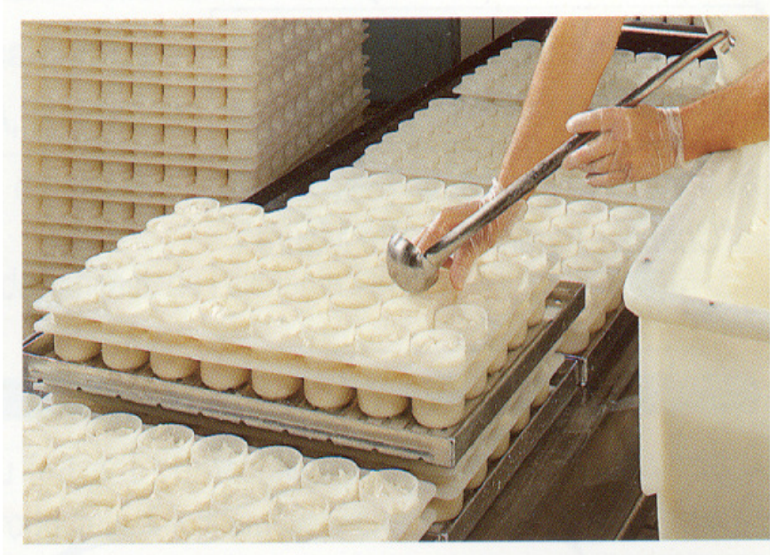
Transfer of soft curd body of goat milk cheese to the plastic hoops for draining whey in a French commercial goat milk cheese plant: (Source: Goat milk cheese plant, Poitiers, France)
