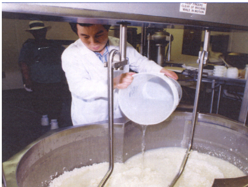
(Washing curds with cold water during Monterey Jack Goat Milk Cheese Manufacture, Fort Valley State University, Georgia, USA)
